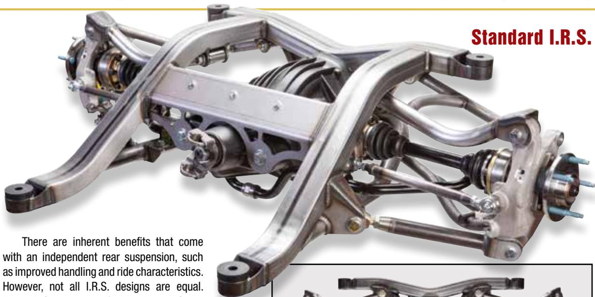
There are inherent benefits that come with an independent rear suspension, such as improved handling and ride characteristics. However, not all I.R.S. designs are equal. Early I.R.S. setups, typified by Jaguar, Cobra and C2/C3 designs have shortcomings when it comes to toe and camber control, limited spindle and anti-squat support, wheel offsets and overall space considerations.
