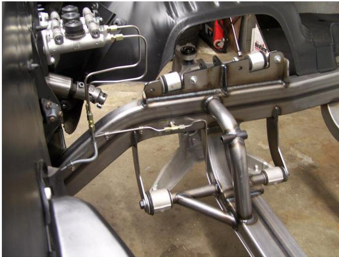
(shown at left), the rear line will need to be modified. Again, minor bends are made to the stock line to fit the new subframe. Stock brake systems can utilize the stock complete rear brake line, but steps should be taken to affix the line to the subframe. If the optional front brake line kit is being used, attach the line with the provided clamps at this time.
