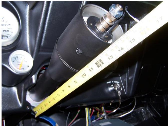
First generation cars will work well with a 32" long steering column. This puts the steering wheel approximately in the same position as a stock column, and provides sufficient clearance between the universal joint and frame rail. To replicate the stock steering column position, place the steering-wheel end 12-1/2" to 13-1/2" from the center of the dash mount fasteners (First gen. only).
