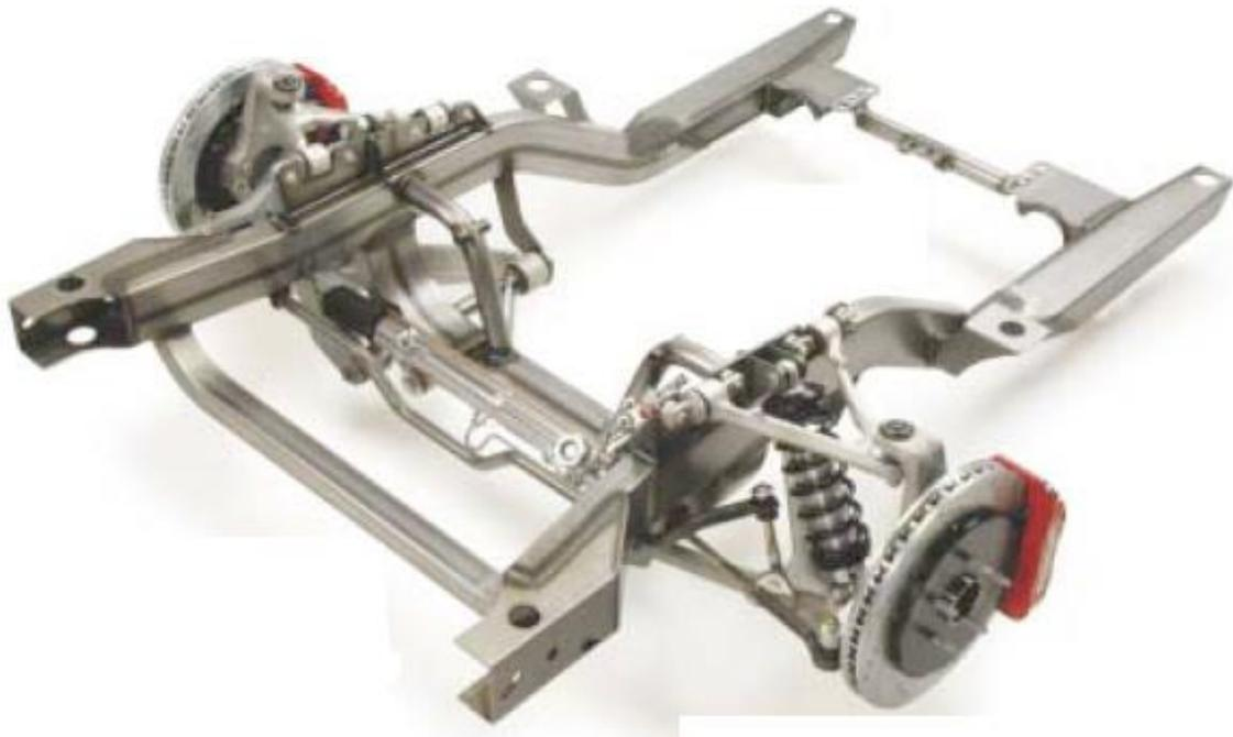
both tie rod boots equally until sufficient clearance is achieved. The tube can also be removed and the boot ties cut to make rotating the boot easier.
