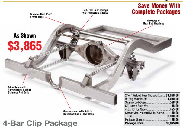
For many applications —especially those with very tight quarters— the 4-bar suspension offers many advantages. Operating on the principle of a "constant motion parallelogram," the design of the 4-bar is such that the rear end housing is always parallel to the ground—pinion angle never changes.
